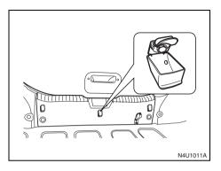
Top strap anchors are located at both sides and at the center of the lower rear tail member in the rear cargo area.
